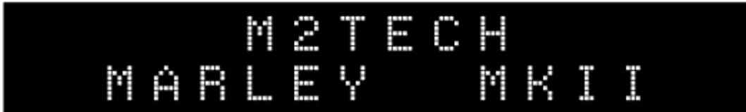
After the activation delay is expired, some general operational information is shown on the MARLEY MKII display: the selected source, the output impedance, the volume level, cross-feed if enabled and the tone control settings. Muting is indicated by the volume level flashing.
