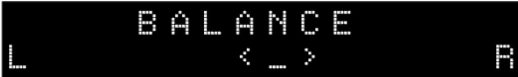
Left channel is increased with regards to right channel by rotating the encoder counter clockwise or by pushing the “arrow left” key on the remote control; right channel is increased with regards to left channel by rotating the encoder clockwise or pushing the “arrow right” key on the remote control.
