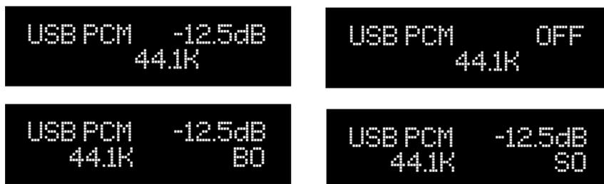
“BO” means “balanced only” and “SO” means “single-ended only”.
