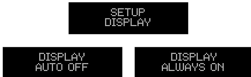
As for the balance, this feature is applied in real-time to give user the possibility to immediately see the results; a short message indicating the present setting appears on the display when the “DIM” key is used.
